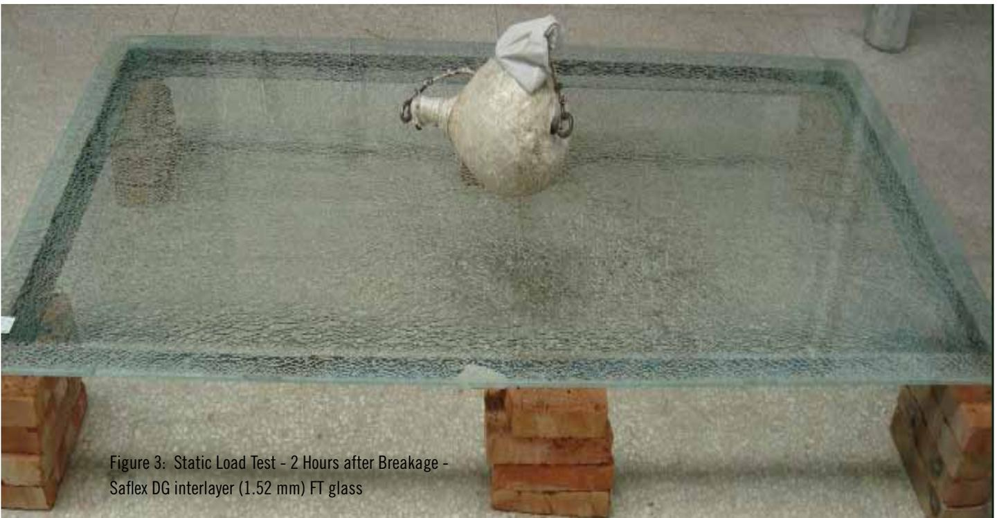
Figure 3: Static Load Test - 2 Hours after Breakage - Saflex DG interlayer (1.52 mm) FT glass
